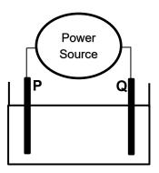
Electrode **P** is the CATHODE of the cell.
