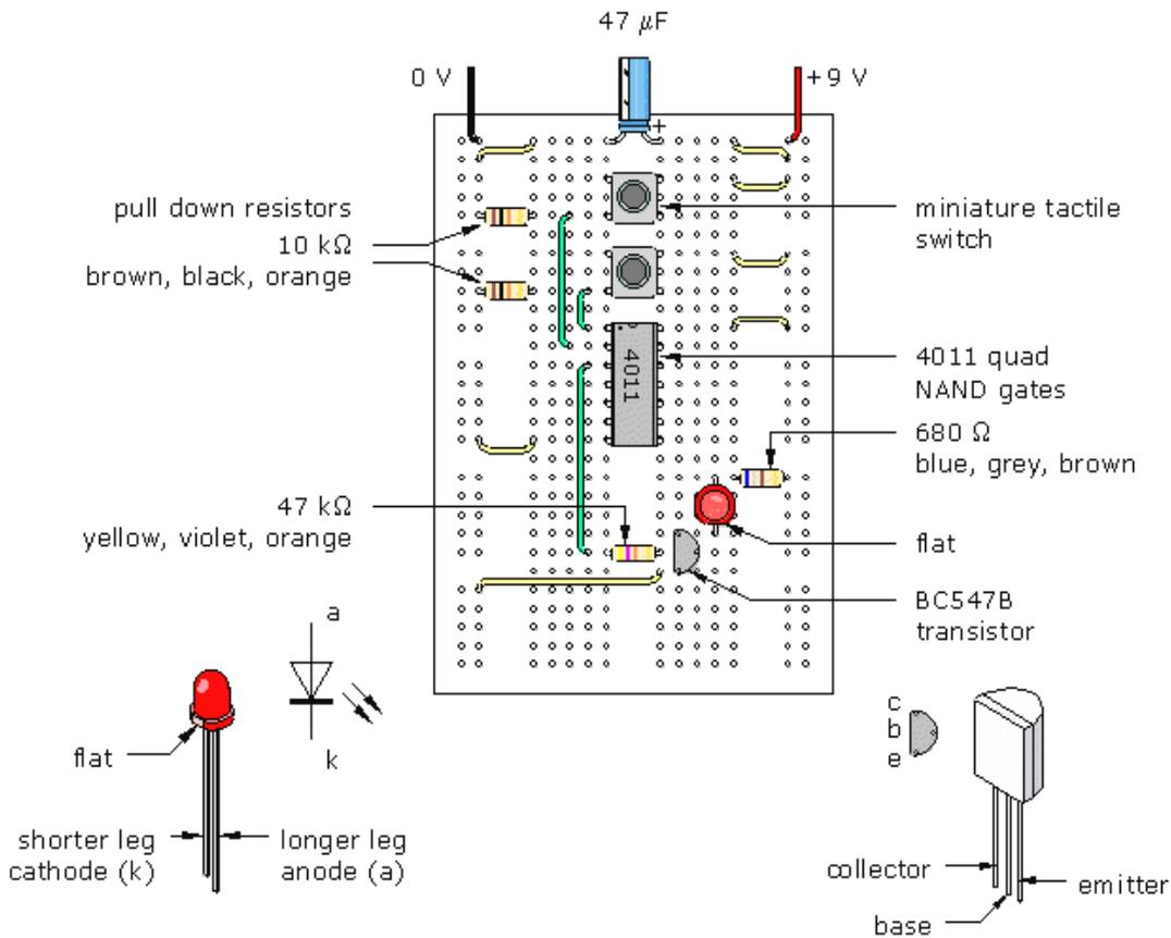
In the prototype circuit, it is not essential to make connections to the unused gates. However, in any final circuit, all unused CMOS inputs must be connected either to HIGH or to LOW. Make it an absolute rule that CMOS inputs are *never* left open circuit.
