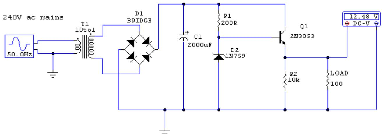
**NOTE:** This circuit above uses a 13 volt Zener diode, D2, which provides the voltage regulation. Approximately 0,6–0,7 volts are dropped across the transistor's b-e junction, leaving a higher current 12,3 volt output supply. This circuit can supply loads of up to 500 mA.
