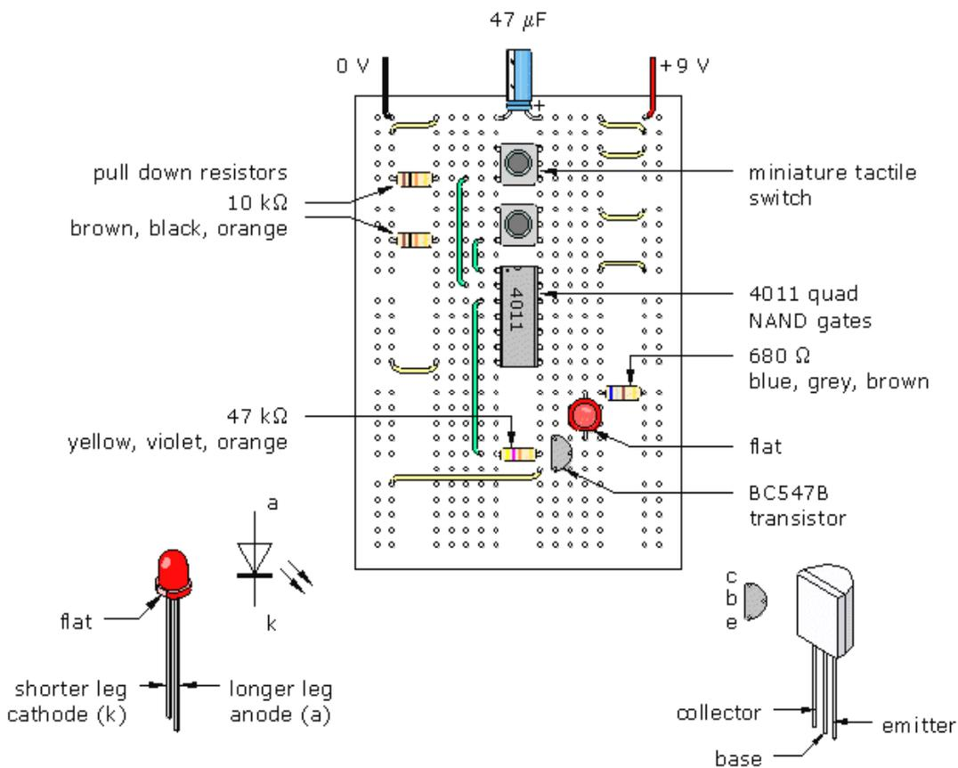
**Proto-board Layout: The NAND gate test circuit**
