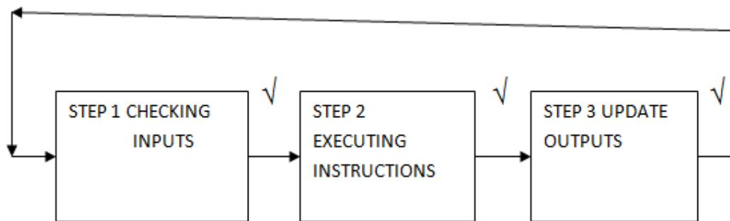
STEP 1: The PLC reads the inputs via the input interface ✓
